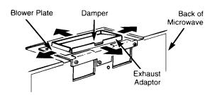
Twist exhaust adaptor to fit under flaps of blower plate. Verify damper moves freely. Square corner on hinge ends.
